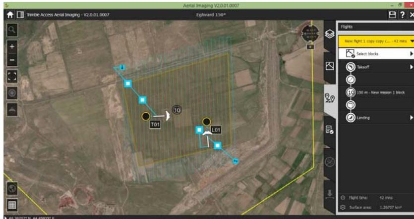
Figure 2. Establishing takeoff and landing points by means of special software
